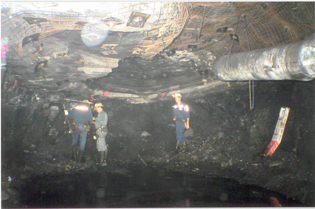
Photo 2 Outburst cavity after cleanup
